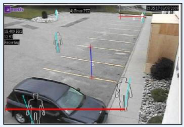
Figure 9. Outdoor Tracking operation mode
