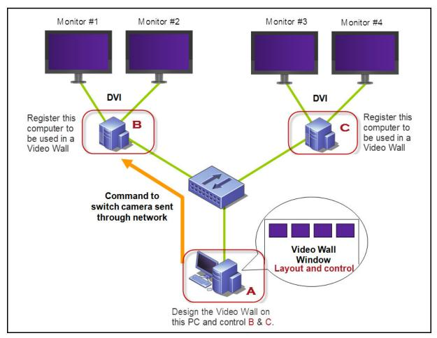
Figure 16. Video Wall setup diagram
