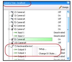
Figure 36. Camera Tree dialog box - Right-click on Hardware Device
