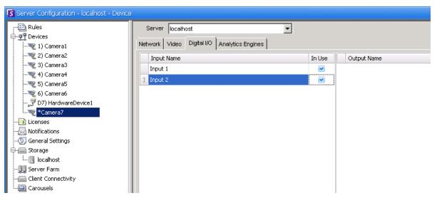
Figure 6. Digital I/O tab for Axis Cameras in Server Configuration dialog box
