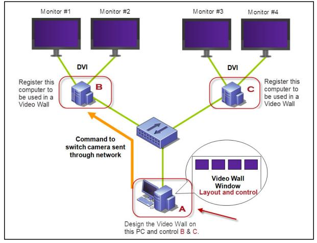
Figure 19. Use computer A to design the video wall
