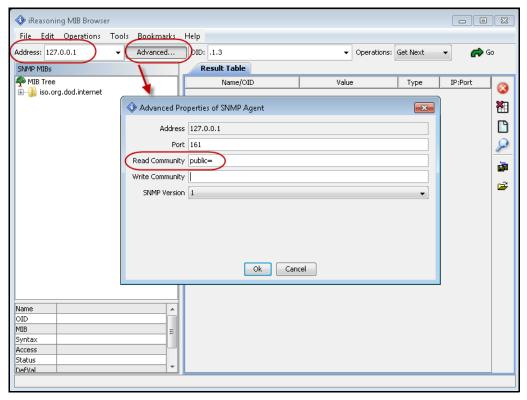
Figure 36. Example using iReasoning MIB Browser with Address field and Advanced options dialog box
