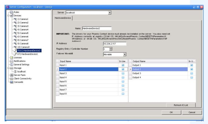
Figure 9. HardwareDevice tab - I/O for Phoenix Devices
