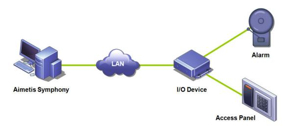
Figure 8. PC sends a signal through the LAN. The I/O device on the LAN receives the signal and then is wired to an alarm in one input or an alarm panel in another input.
