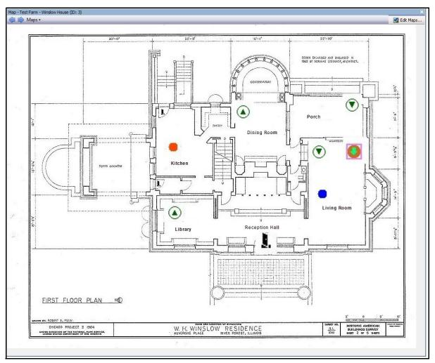
Figure 33. Example of a typical map with camera, PTZ camera, digital I/O, and control access device icons, and rules
