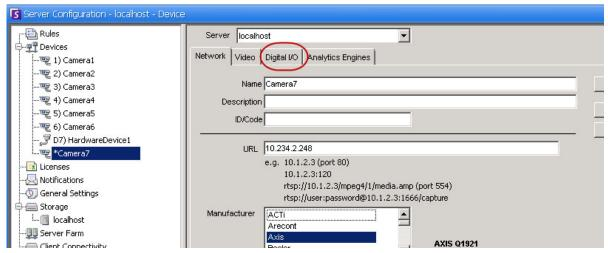
Figure 5. Adding an Axis Camera with Digital I/O invokes a Digital I/O tab in the Server Configuration dialog box
