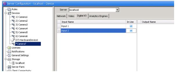
Figure 39. Digital I/O tab for Axis Cameras in Server Configuration dialog box
