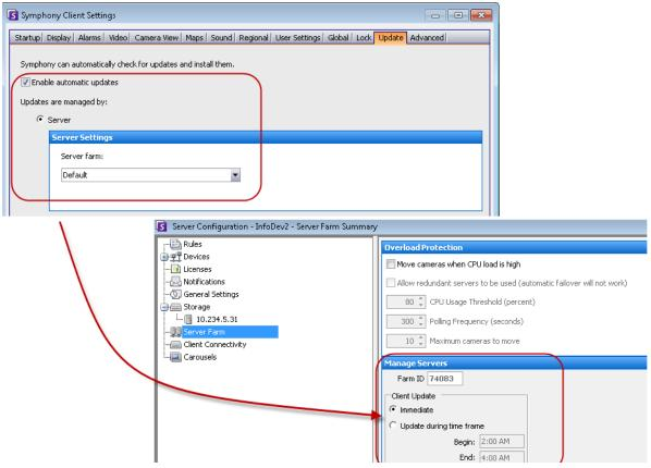
Figure 3. Device Pack Update Installations Managed by Server - Example
