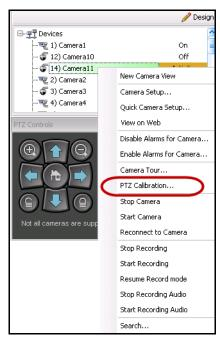
Figure 26. Right-click on PTZ camera for PTZ Calibration option
