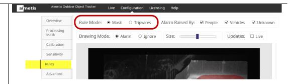
**IMPORTANT**: The **Trigger** event selected in the Axis camera setup interface MUST match the **Rule Mode** configured in the AOOT interface.
